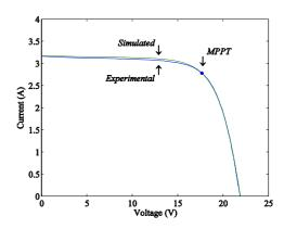
Fig. 1. I-V simulated and experimental curves at STC.
