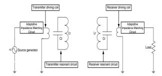
Fig. 1. WPT via strongly coupled magnetic resonance.
