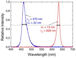
Fig. 3. Output spectra of the red and blue chips.
