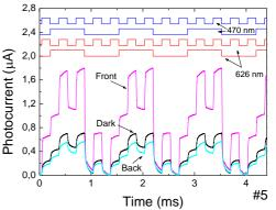
Fig. 4. Photocurrent measured without and under front and back optical bias when the device is at the central position.
