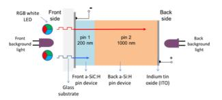
Fig. 2. Simplified cross-section view of the photodetector.
