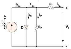
Figure 1 – Equivalent circuit of a solar cell.
