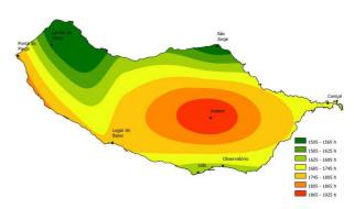
Figure 4 - Equivalent sun hours at peak power in Madeira.
