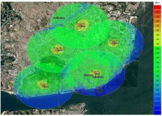
Fig. 3 – Coverage with model Okumura-Hata.
